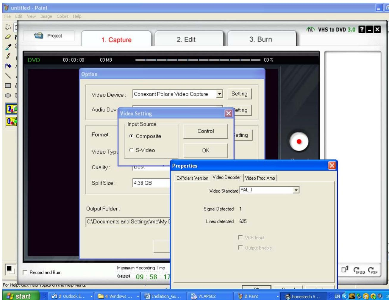
4) Audio device setting: You **DO NOT** need to choose any audio device since the chipset for our VCAP602 has combined video and audio together and the audio recording will be controlled by the video device.
